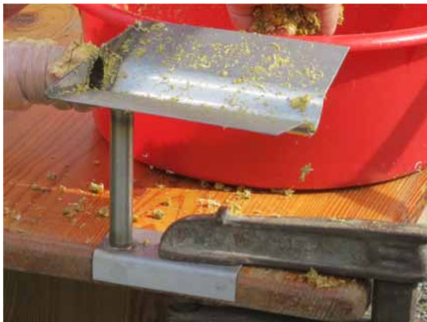
Picture 3-6: Funnel used to stuff chamomile, fixed on the table using a clamp
